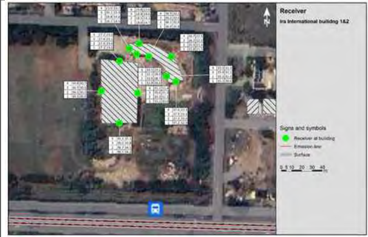
Noise levels at different floors (at different sides of building) at Ira International School
