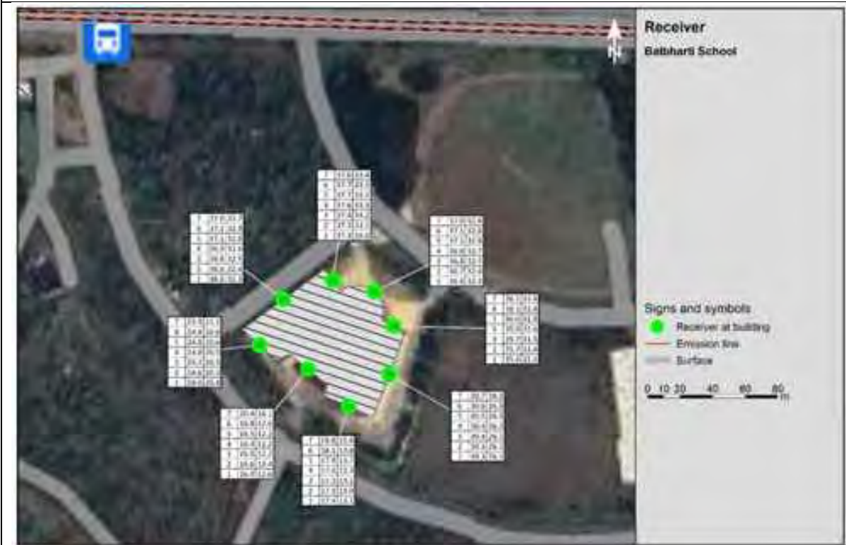
Noise levels at different floors (at different sides of building) at Balbharti School
