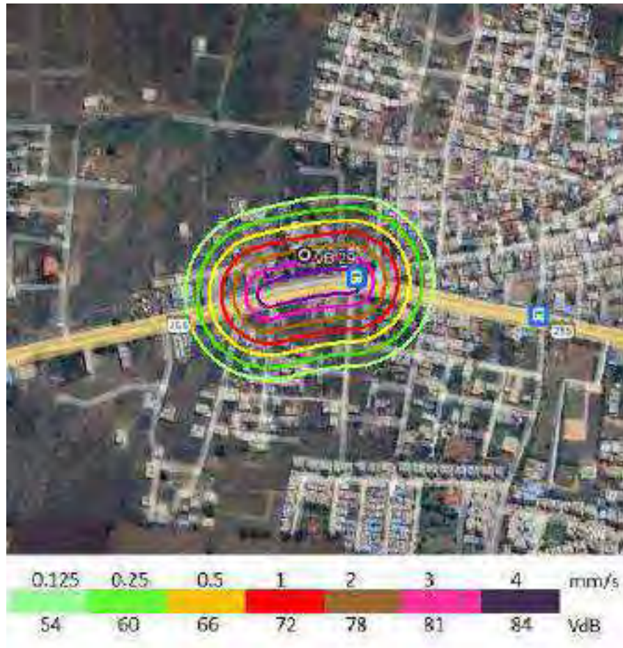
Figure 4.6: showing the predicted vibration contours due to train operation at Rural Hospital Hingna
