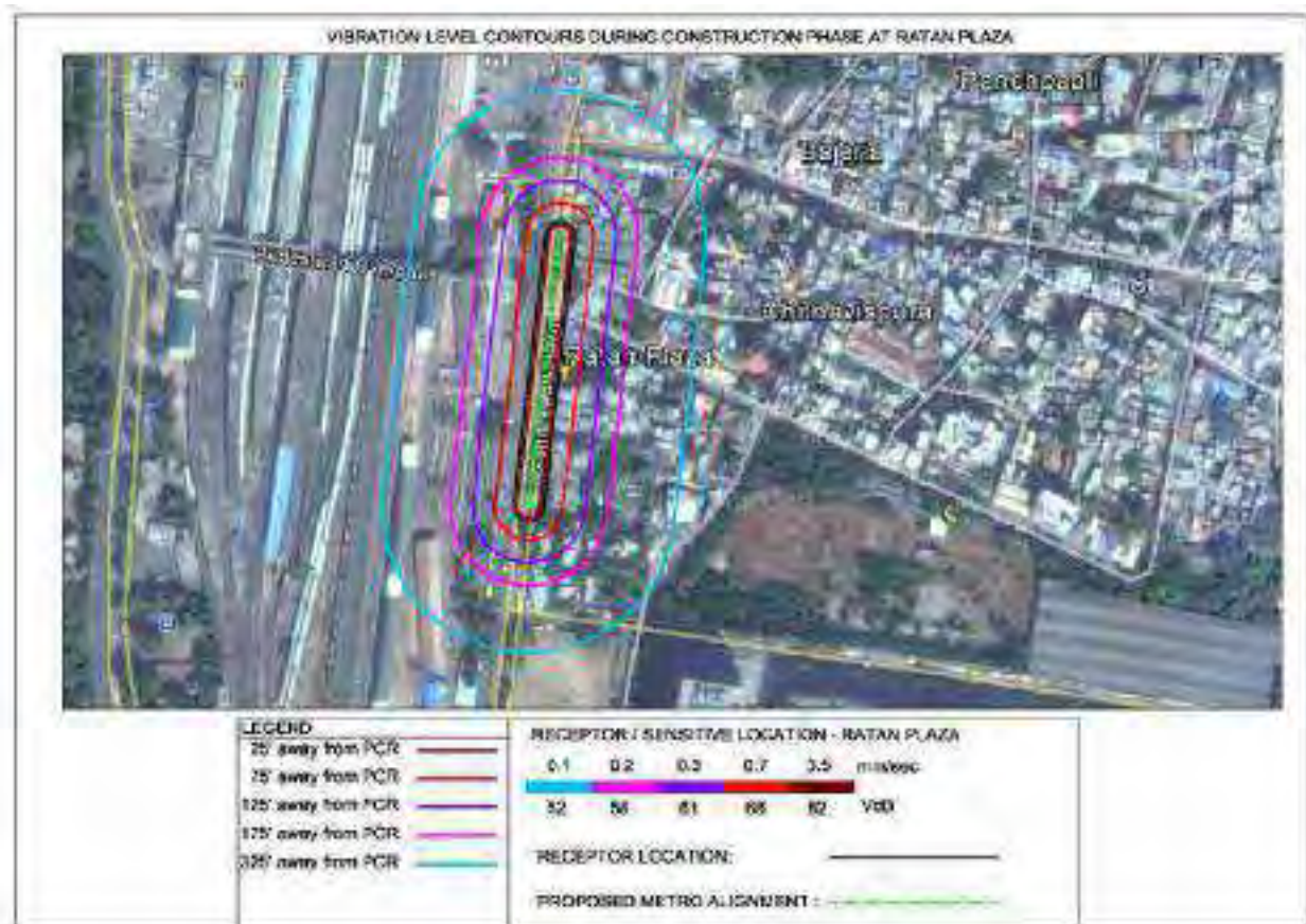
Figure -6.19: Vibration level Contours during construction phase at Rattan Plaza
