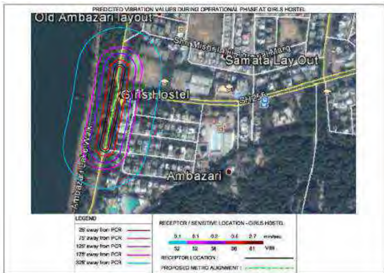
Figure 6.41- Predicted vibration values during Operation Phase at Building Near Ambazari Lake
