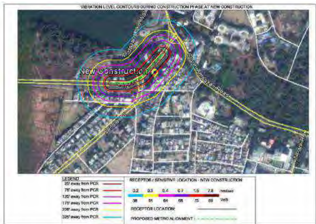
Figure -6.23: Vibration level Contours during construction phase at New Construction in Subhash nagar
