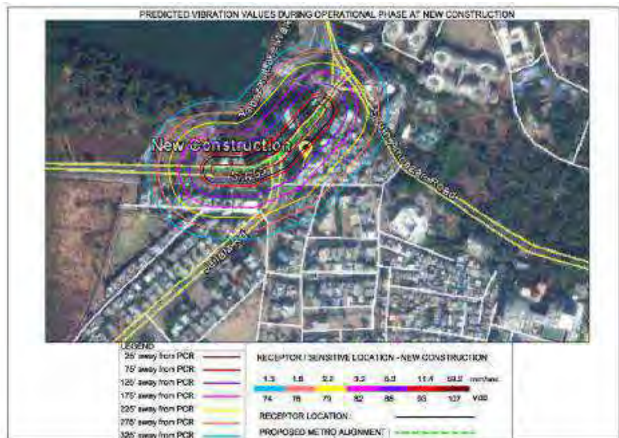
Figure 6.42- Predicted vibration values during Operation Phase at New Construction in Subhash nagar
