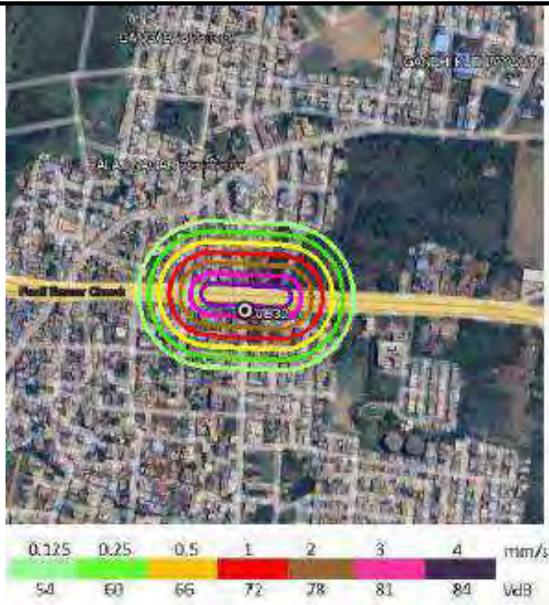
Figure 4.9: showing the predicted vibration contours due to train operation at Pardi residential area.
