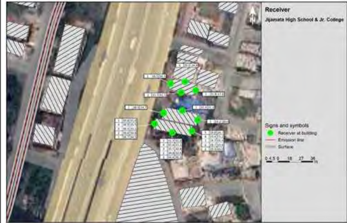
Noise levels at different floors (at different sides of building) at Jijamata High School and Jr. College
