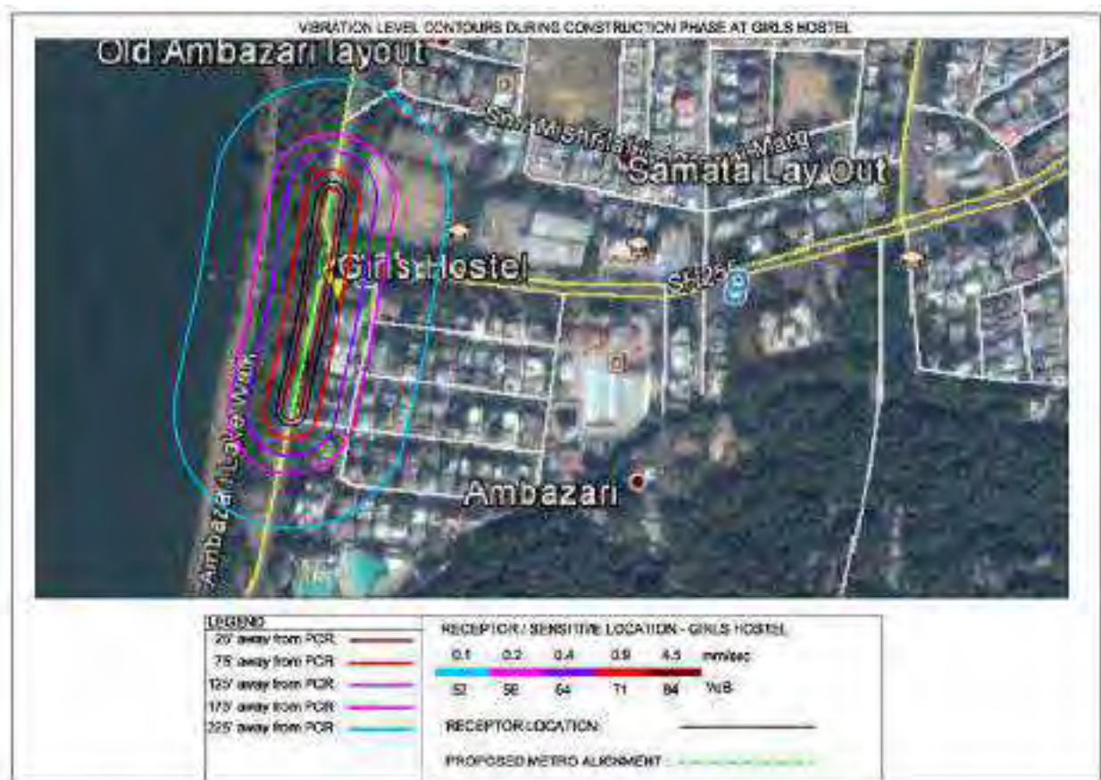
Figure -6.22: Vibration level Contours during construction phase at Building Near Ambazari Lake
